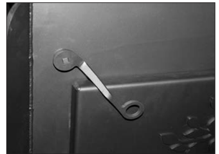
The bypass lever interlocks with the door when the combustor is engaged (bypass closed). This safety feature makes it impossible to open the loading door without opening the bypass.
