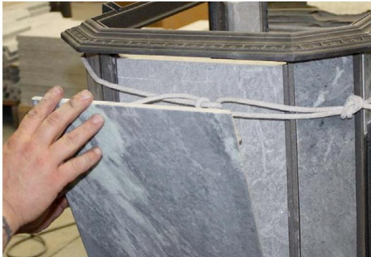
10. The replacement stone will rest on two pieces of flat gasket. The gasket should be placed on the slightly raised part of the stove base.
