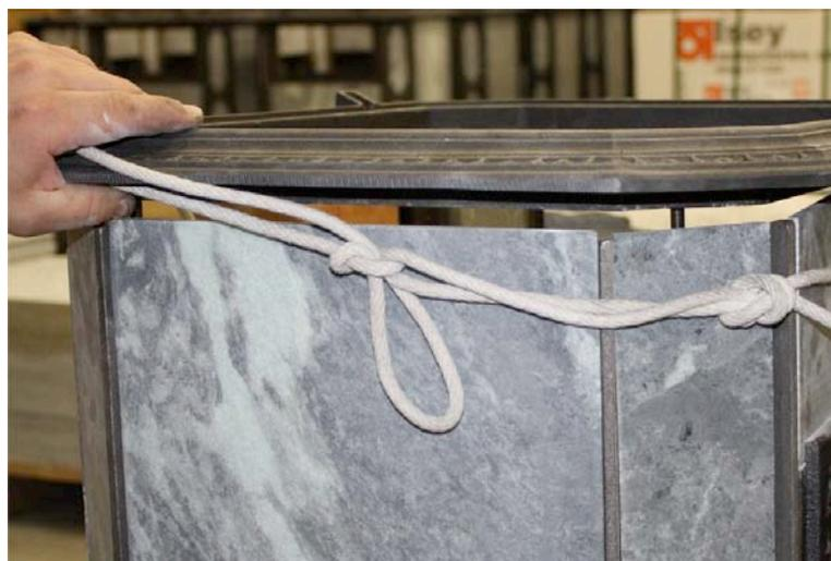
13. Re-install the corner castings one at a time. Place the bottom edge into the base first, then lift the top frame enough to get the top edge of the corner casting in place. When the top frame is properly seated it will cover the top edges of all four corner castings.
