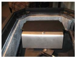
3. The hood is held in place with two bolts and nuts. To remove the bolts use a ½" socket from inside the firebox and wedge a flat blade screwdriver between the hood and the nuts inside the top of the stove. It may be helpful to spray penetrating liquid on the nuts. (The nuts do not need to be replaced after the new combustor is installed, simply drop the bolts back through the hood for proper alignment).
