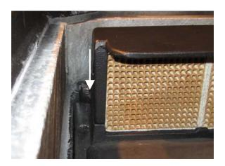
4. Gently lift the hood from the stove. Turn it upside down to remove the old combustor. Use a putty knife and vacuum to remove any residual gasket material from the hood as well as the area where the combustor rests on the baffle plate.
