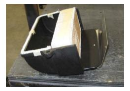
5. The replacement combustor is pre-wrapped in a white gasket material as well as a stainless steel band. Place the new combustor on the baffle plate to the right of the rectangular opening to the firebox. The small metal strip welded to the stainless band on the combustor should
