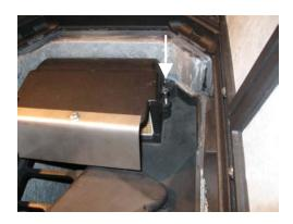
7. Replace the top lid on the stove. Be sure it is seated properly on the gasket.
