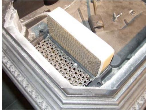
7. Place the cast iron hood over the combustor. The combustor may seem a little loose at first, but the white gasket material will expand upon heating. Use the bolts for proper alignment. It is not necessary to re-install the nuts on the bolts.
