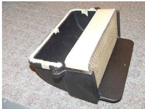
6. The replacement combustor is pre-wrapped in a white gasket material. Place the new combustor on the baffle plate to the right of the rectangular opening to the firebox.
