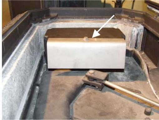
4. The hood is held in place with two bolts and nuts. To remove the bolts use a 1/2" socket from inside the firebox and wedge a flat blade screwdriver between the hood and the bolt head inside the top of the stove. It may be helpful to spray penetrating liquid on the nuts inside the firebox. (The nuts do not need to be replaced after the new combustor is installed, simply drop the bolts back through the hood for proper alignment).
