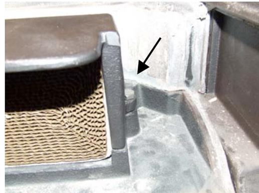
5. Gently lift the hood from the top of the stove. Turn it upside down to remove the old combustor. Use a putty knife and vacuum to remove any residual gasket material from the hood as well as the area where the combustor rests on the baffle plate.
