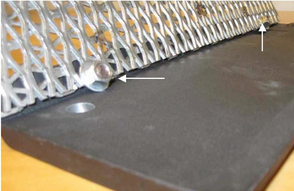
19. Place the scoop with the expanded metal upside down, with the sharp edge down, on a hard surface such as cement floor. Use the heel of your foot to apply pressure on the parts to bend the expanded metal outward so that the angle is not as sharp.
