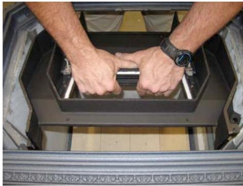
10. Remove the air guide (W-172) from the front edge of the new combustor pan. It is held in with two bolts and two washers.
