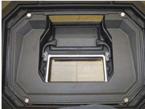
6. Using a 9/16" socket remove the two nuts from the two eyebolts that hold the combustor to the vertical supports (under the combustor pan) and remove the eyebolts by tilting the eye off from the supports and pulling them downward.
