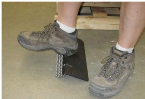
20. Slide the new scoop into the lip of the combustor pan and then slide it inward so that it sits into the two fingers. If the scoop will not go in easily it may be because the expanded metal is hitting the two bolts that fasten the cast air chute above the scoop.
