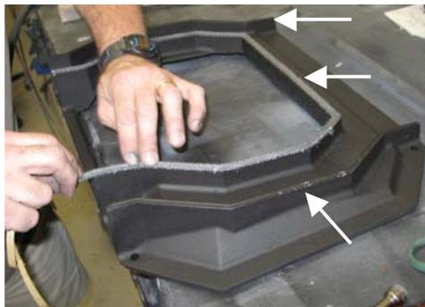
23. Install the air duct cover to the comb. pan. Move the cover as needed to align it with the pan.
