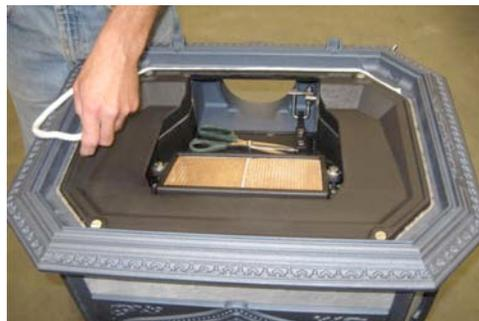
29. Recheck that the 1/4" gap has been maintained between the glass and air guide.
