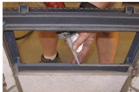
12. Place 1/4" gasket on top of the cement on the *Comb. Pan*. Hold it on with two pieces of masking tape. Otherwise it will fall off when it is turned right side up.
