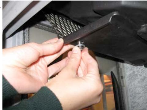
21. Fasten the scoop to the single fingered support with the bolt and washer.
