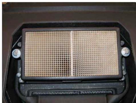
4. Detach the bypass lift guide (W-178) by removing the two bolts that attach it to the top side of the bypass door (W-253). You will need a 1/2" wrench or socket.
