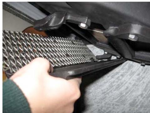
9. From the top of the stove place one hand through the combustor port and pull the combustor pan (W-160) up and out of the stove.
