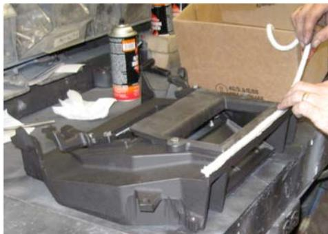
13. Reach inside the firebox and apply a generous bead of cement on the two seams on each side of the rear frame. This seam is where the vertical supports abut the rear frame.
