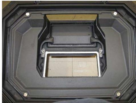
25. Replace the old cement on the flue collar with new. Replace old gasket with gasket from bag "A". Apply cement around the perimeter of the rear frame on the inside of the bolt holes where the rear frame will meet the flue collar. The bottom does not get cement.
