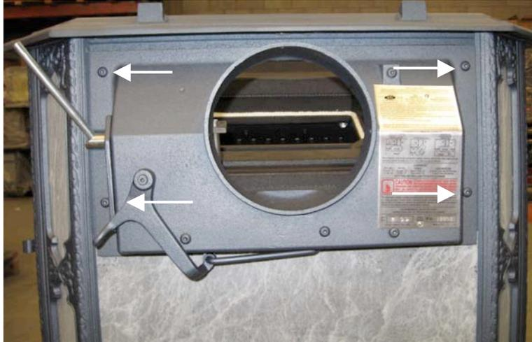
8. Reach into the firebox and remove the combustor scoop (W-249) and metal diffuser (W-305) by removing the single bolt that attaches it to the combustor pan scoop support (1/2" wrench or socket to loosen). Carefully slide the scoop toward the loading door and forward to completely release it. **Be very careful with the metal diffuser it is extremely sharp around the edges.**
