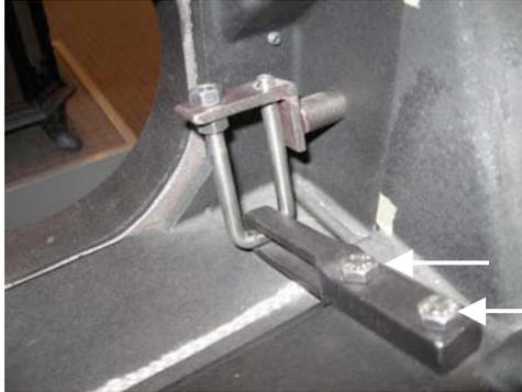
5. Using the large flat blade screwdriver, remove the four bolts that hold the top half of the combustor assembly (air duct cover, W-163). Make a note of their positions as all the screws are not the same length. Lift the cover up and off the assembly.
