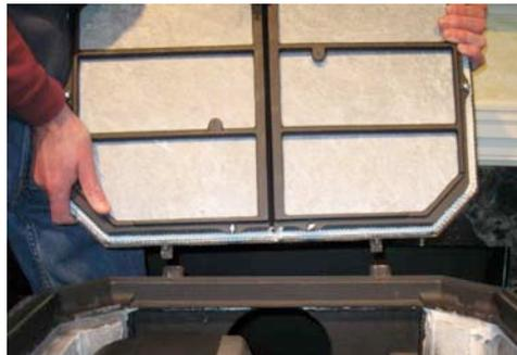
3. Using a 1/2" wrench or socket, remove the two bolts and washers that hold the combustor cells and combustor frame (W-165/166) in place. (These bolts do not need to be reinstalled as they are for transport only).
