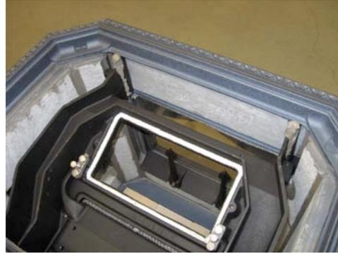
18. If you are transferring your existing expanded metal diffuser than carefully remove the fastening nuts and bolts and reinstall on the new scoop. **BE VERY CAREFUL! THE EDGES ARE EXTREMELY SHARP!**
