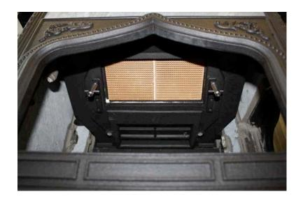
6. Slide the back edge of the replacement scoop into the lip of the bypass frame. If there is any gasket under the front of the bypass frame, remove it. Raise the front edge and guide the holes in the scoop over the posts. The top of the screen should touch the top of the firebox. Be sure the screen clears the air guide at the top front of the firebox. You may need to push in on the screen slightly to have it clear the air guide.
