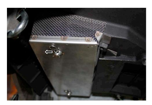
8. Once the proper fit is achieved remove the scoop and tighten the lock nuts with a ½" wrench. It will be helpful to hold the supports in place
