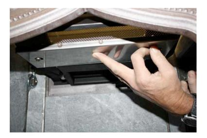
7. Adjust the posts so the holes for the hairpin cotter pins are facing the loading door for easy access. Once the hairpin cotter pins are in place there should be very little up and down movement from the scoop.
