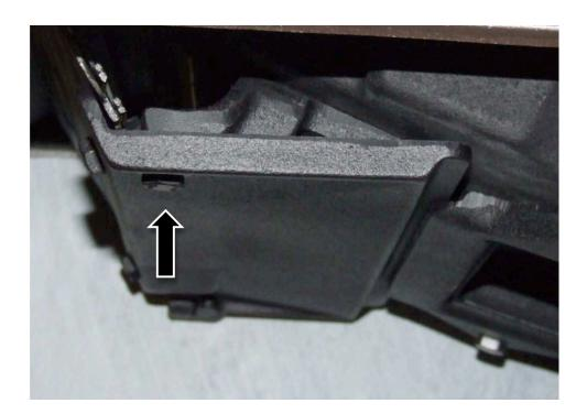
4. Use a 1/2" socket or wrench to remove the two scoop supports from the top of the firebox. Each support is fastened with two bolts. The new scoop posts will replace the existing hardware and supports.
