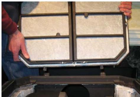
3. Remove the catalytic combustor from the stove. If you have not already done so remove the transport bolts with a ½” socket or wrench. The bolts do not need to be returned to the stove. Lift the combustor out of the stove.
