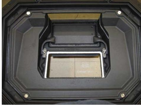
4. Remove the gasket from around the combustor opening in the combustor pan. Use a putty knife and wire brush to remove any residual gasket or glue. Vacuum up any loose debris.
