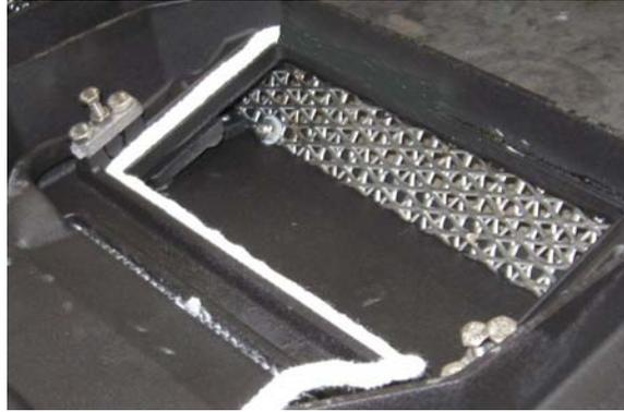
8. Return the catalytic combustor to the stove. The open side of the hooks for the transport bolts should face the flue exit of the stove. (Do not reinstall the shipping bolts.)
