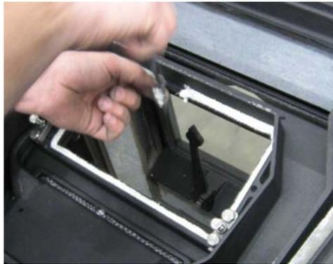
5. Dry fit the replacement gasket. Start in a corner and lay the gasket into the channel until you are back to the starting point. Cut off excess gasket if necessary with sharp scissors. Set gasket aside.
