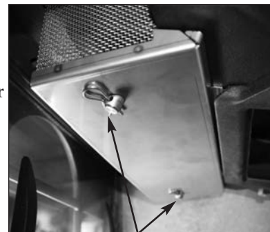
Pull the two cotter pins on the underside of the scoop plate to remove the screen/plate assembly from the stove for cleaning.
