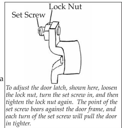
*To adjust the door latch, shown here, loosen the lock nut, turn the set screw in, and then tighten the lock nut again. The point of the set screw bears against the door frame, and each turn of the set screw will pull the door in tighter.*
