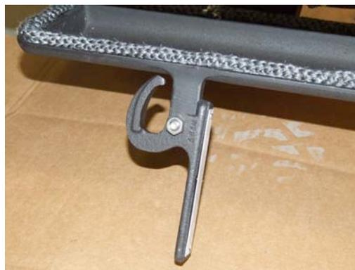
4. Tighten the bolt so that the handle moves with some resistance and then secure it in place with a 1/4-20 nut. Hold the bolt still using a 7/16" wrench while tightening the nut so that the tension on the handle is not changed.
