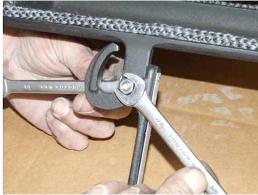
5. Be sure the handle moves along with the bolt and nut freely.
