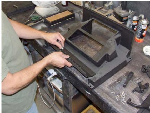
16. Remove the two bypass cover retainers from the original pan. These are the gray cast iron parts at each side of the bypass cover pivot points. First remove the center “adjustment” screws from each retainer (7/16” wrench) and then remove the two bolts on each retainer (1/2” wrench).
