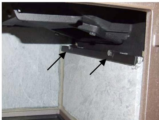
8. While inside the firebox locate the 2 bolts on the backside of the doorframe. Loosen the locking nuts clockwise, then turn the mounting bolts counterclockwise, using a 1/2" wrench, to release them from the combustor pan.
