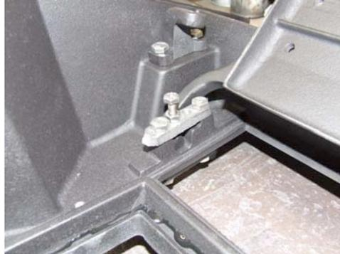
23. Apply gasket glue along the channel around the combustor assembly port and insert 1/4" gasket along the channel, with the split in the gasket at any of the four corners.
