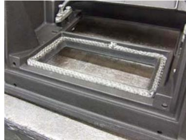
21. Place the bypass cover into position and install the bypass retainers with the four 1/2" hex head screws. Notice that the bypass retainers are not identical. The two center holes should be offset toward the outside of the pan and the smaller of the two holes should be toward the bypass cover as seen below.
