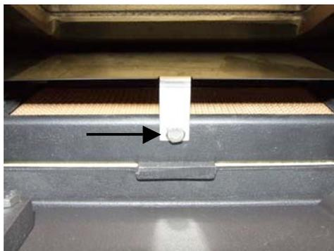
3. Remove the catalytic combustor assembly by removing the two shipping bolts (if they are still in place) and lift the combustor out. The bolts are found at each end of the combustor assembly and require a 1/2" wrench. Once the bolts and flat head washers are removed, lift and turn the assembly 90° and pull it out the rear vent hole. (The two 2-1/2" bolts are only necessary for shipping and do not need to be reinstalled. Leaving them out makes it easier to remove the combustor for cleaning.)
