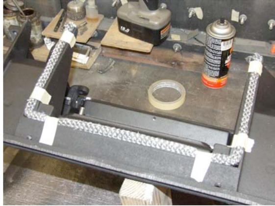
27. Apply a small bead of gasket glue across the bottom edge of the elongated rear wall of the new combustor pan, which will rest on the exterior rear stone when the combustor pan is installed.
