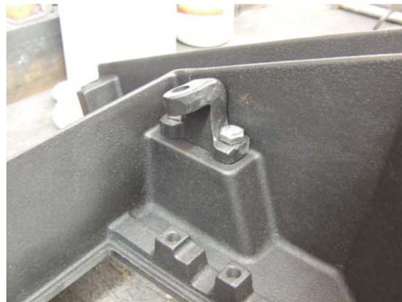
15. Transfer the air chute from the original pan to the new one, but do not tighten the bolts completely as the chute will have to be adjusted after the pan is installed. The air chute is the long cast iron plate that protrudes from the front edge of the combustor pan and is fastened with two bolts and two flat washers that come up through the bottom side of the chute and into the bottom side of the front edge of the combustor pan.
