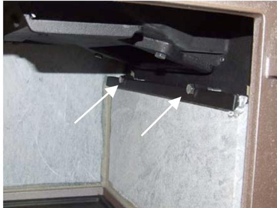
38. Use the shank of a 1/4" drill bit as a measuring device to reset the space between the front edge of the air guide and the glass panel. The spacing should be adjusted so that the drill bit may move between the two with just a slight bit of friction. Tighten the two air chute bolts securely with the proper 1/4" spacing.
