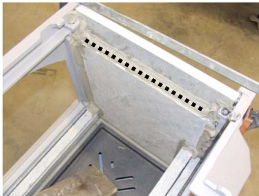
32. Loosen the clamp, or rope, for this step, and then retighten afterward. Holding the combustor pan in the center, lower the pan into place. Watch the sides of the pan so that the stone panels do not get hit and chipped.
