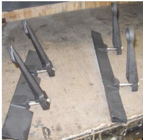
2. Spray a lubricant or penetrating oil on both of the bolts that attach the glass andiron(s) to the backside of the front casting (WD-40, Break-Free CLP, Kroil, PB Blaster,etc). Let it work on the bolts for up to 24 hours. Re-apply as necessary. Direct the spray under the retainer where the bolt passes through to the front frame
