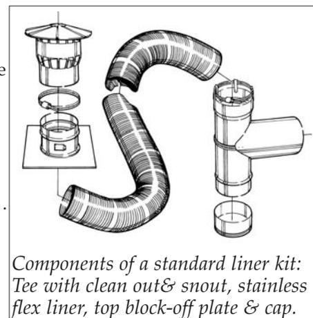
*Components of a standard liner kit: Tee with clean out & snout, stainless flex liner, top block-off plate & cap.*
