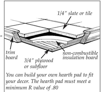
**\*The R Value of the hearth pad can be reduced down to 0.40 with the use of the Progress Hybrid Ash Lip EXCEPT WHEN USING THE SHORT LEGS.**
