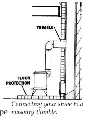
**B. Build a solid brick surround around a tile liner** - Frame a 3.5" thick brick surround into the combustible wall you need to pass through. Maintain a minimum 12" brick separation from the clay liner to combustibles. The minimum 5/8" thick clay liner should be cemented in place and run from the outer surface of the brick to the inner surface of the chimney. (See Diagram B Below)
