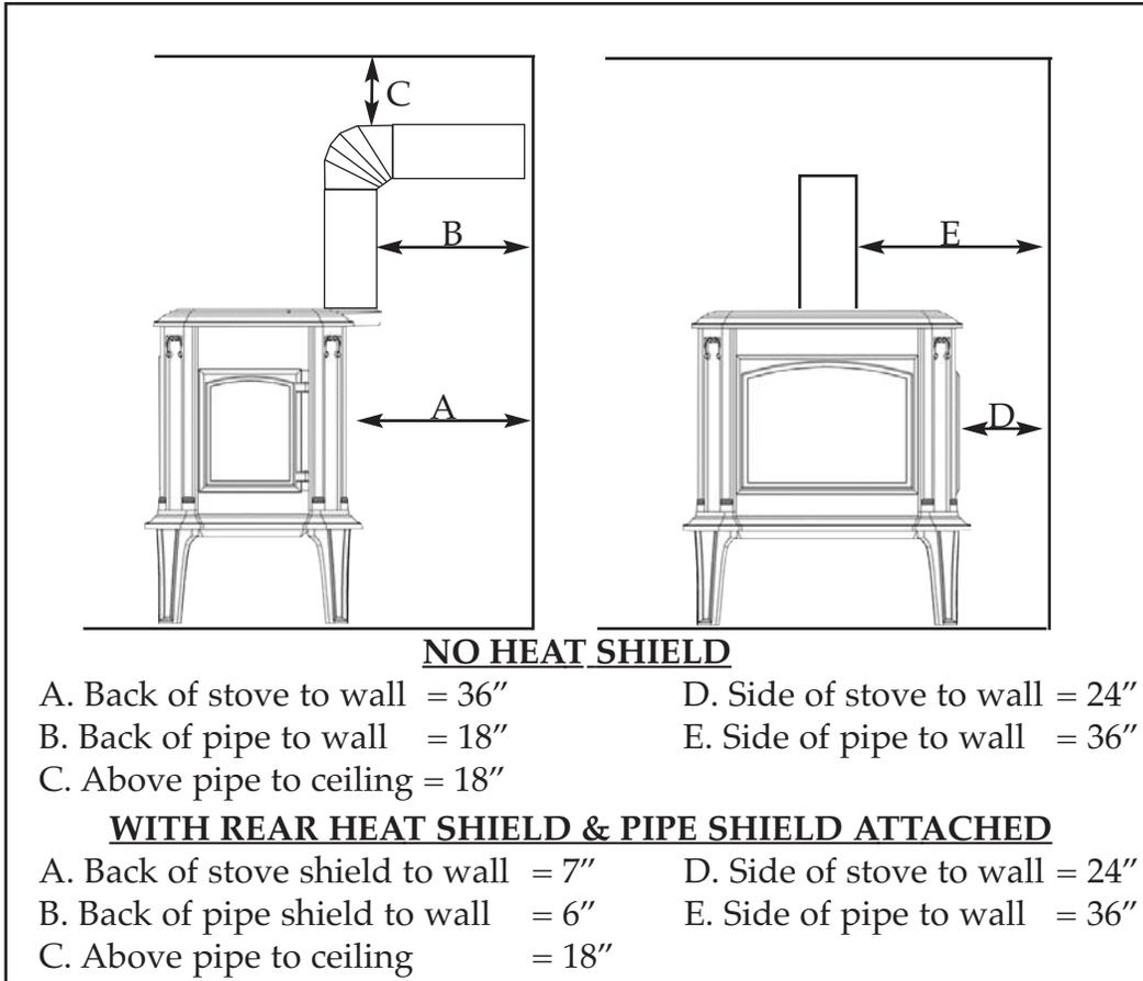
**2) Parallel Installation, Single Wall Pipe, Back Vent**
