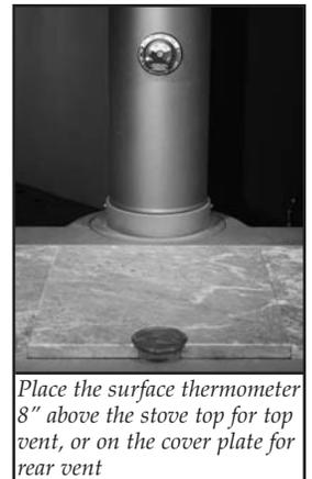
Place the surface thermometer 8" above the stove top for top vent, or on the cover plate for rear vent
