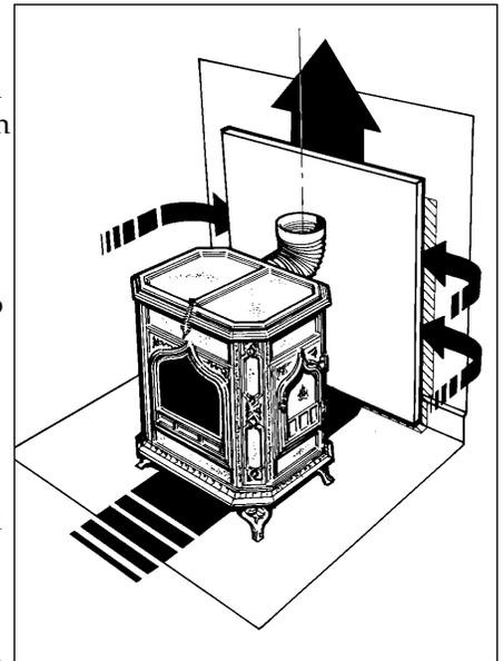
*Wall shields should be open on at least three sides to allow for air flow.*
