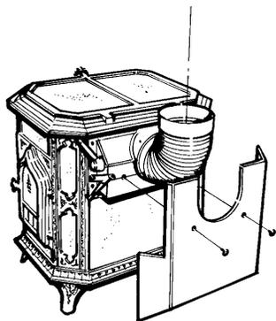
*Rear heat shields are unobtrusive, and attach to easily to the back of the stove.*
