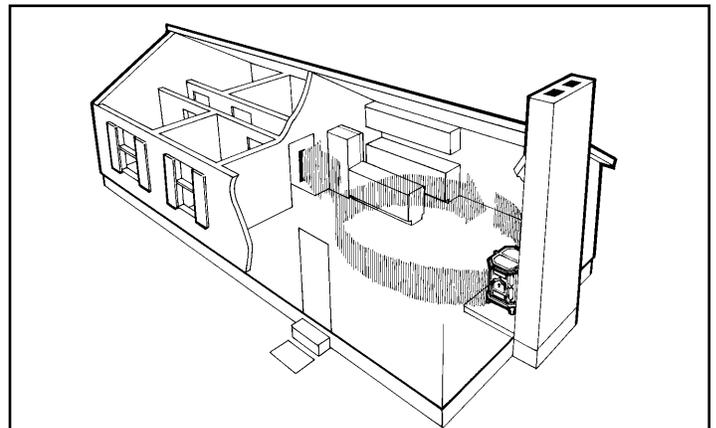
*Moving heat down long hallways and into the rooms furthest from the stove is more difficult. Sometimes cold air returns or doorway fans can help.*
