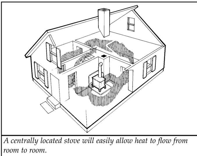
*A centrally located stove will easily allow heat to flow from room to room.*
