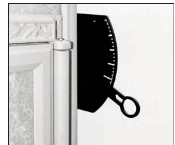
The amount of combustion air available in the firebox is controlled by the damper lever. (Fig 2)
