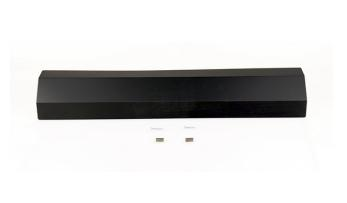
The pipe shield is designed to reduce the required clearance from the pipe to combustibles, please consult your owner's manual for approved clearance reduction. If your installation includes a  $90^{\circ}$  elbow, the shield must cover the area of the elbow that is parallel to the combustible behind it. The pipe shield may be cut to length as needed for your specific installation.
