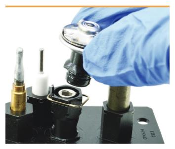
Beneath the round hood is a one-piece pilot orifice, which can be removed with a 5/32 hex wrench. Gently insert the hex wrench and unscrew the pilot from the housing. Lift the pilot out of the housing.
