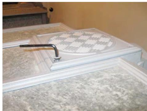
6. It will be helpful to disconnect the lift guide from the bypass cover for better access to the gasket channel. Use a ½” wrench to loosen the bolts. Prop the bypass door open. Dry fit the gasket in the channel and trim to fit if necessary. Place gasket glue into the channel. The break in the gasket should go in the center of the long length closest to the front of the stove. Re-connect the lift guide to the bypass cover.
