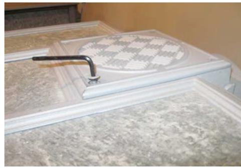
9. Replace the combustor scoop and diffuser. Place the far end of the scoop onto the support at the top of the firebox. Angle the back edge of the scoop into the lip of the bypass frame. Using (1) 5/16"x3/4" bolt fasten the scoop to the support closest to the loading door.
