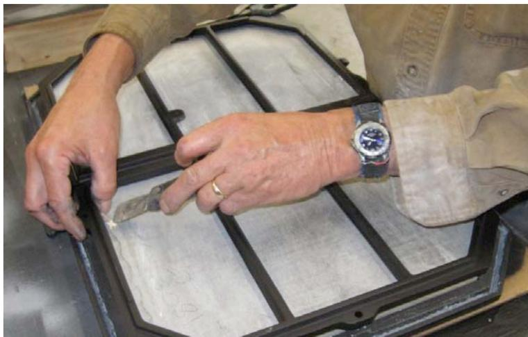
12. Tighten the screws evenly. Give each screw a few turns and repeat around the frame. Tighten the screws snugly, but do not over-tighten as this may lead to broken stone. With the screws completely tight you should be able to squeeze the retainer toward the lid and have no visible motion.
