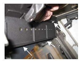
14. Replace the combustor scoop and diffuser.
