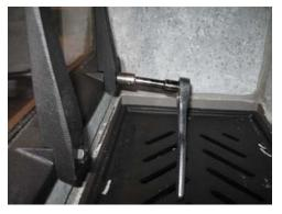
13. Confirm there is a 1/4" space between the interior glass panel and the air guide. A 1/4" drill bit (or #2 pencil) is helpful to check the gap. The air guide is at the top front of the firebox. If adjustment is necessary, slightly loosen the two air guide bolts, using a 7/16" socket, move the air guide, then retighten.
