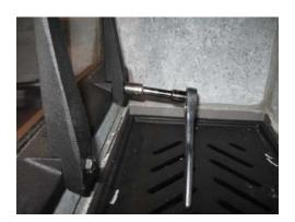
4. Remove the two upper window clips using a 7/16" socket or wrench.
